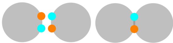
FIG. 1. Simple 2D model for self-assembly of building blocks with rotational degrees of freedom. The two identical monomers form a dimer when the orange and cyan patches overlap.
